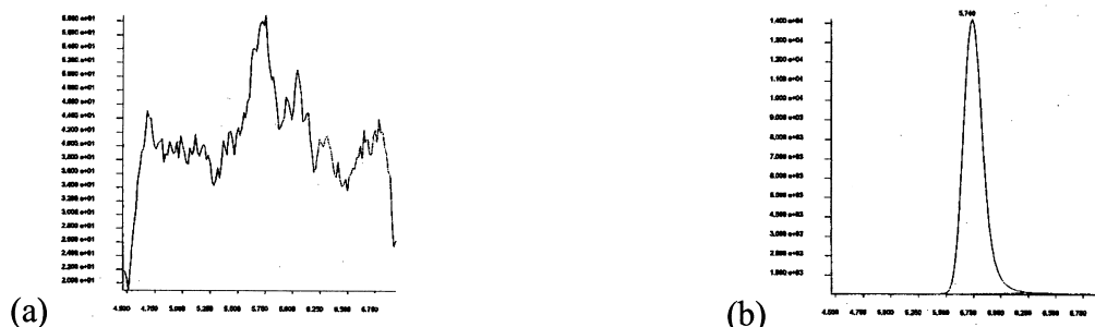
Fig. 3. Typical chromatogram obtained from a blank plasma sample spiked with 10 ng/ml of SCG. (a) I.S.; (b) SCG.
